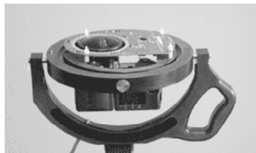
Fig. 2. Self-leveling mount system for hemispherical photograph acquisition with the top of the camera oriented north.
